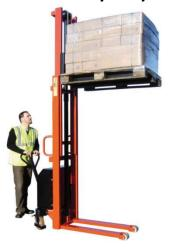
Battery powered lift, manual traction
